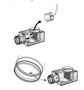
Figure 3. ALS. Damper removal.
