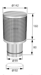
Figure 4. DCC. Unit of measure = mm. Weight: 1.2 kg. Cutout dimension = Ø102 mm.
