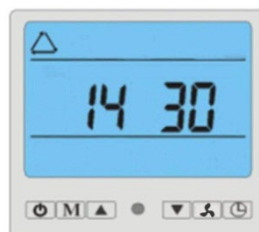
Picture: Parameters check, input water temperature 30°C.
