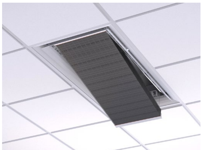
Figure 16. Removing the face plate and folding out the coil for accurate cleaning in the event of high hygiene requirements. Note! requires the product to be ordered with the accessory, fold-out coil, and that flexible connection hoses are used on the water side.
