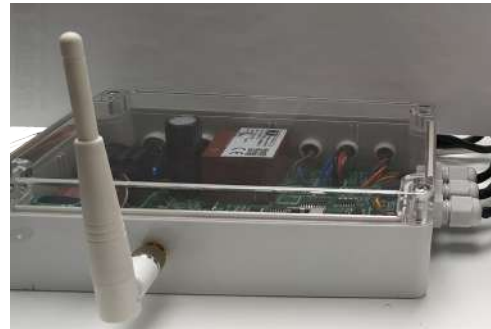
WIFI antennae position during use – please direct the WIFI antennae upwards to ensure signal quality
