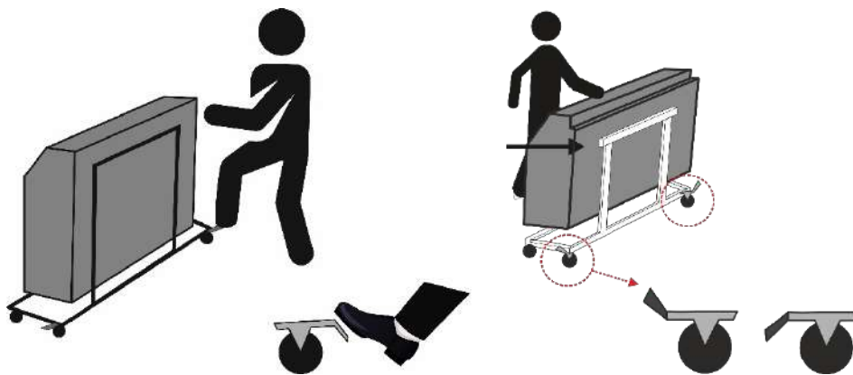
Obr.1 After moving Athmoss on the mobile stand to the application site, secure the wheel brake (locking). The wheel brake is locked when the brake lever is down. The wheel brake is released when the lever is up.
